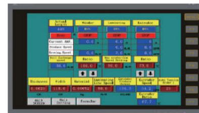
PLC program with a user-friendly HMI touchscreen interface, interlocking operation of all units and data memory as optional.
