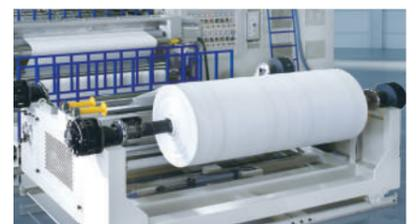
Unwinding unit configures with missing fabric detection and automatic unwinding change device; not only running with magnetic brakes, pneumatic disc brakes can be used as optional.
